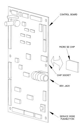
**Figure 3.1 Control Board Components**
