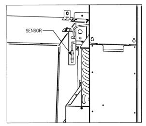
Figure 8.3 Temperature Sensor
