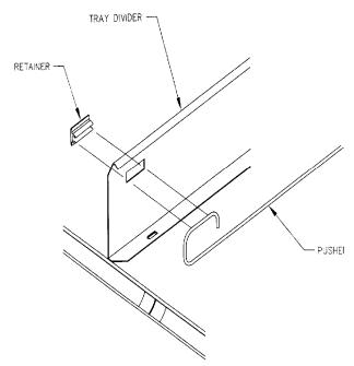
Figure 5.3 Pusher Bar Installation
