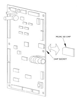
Figure 8.1 Loading Control Software
