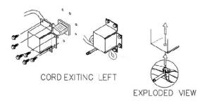
Figure 8.4 Power Cord and Protective Cover
