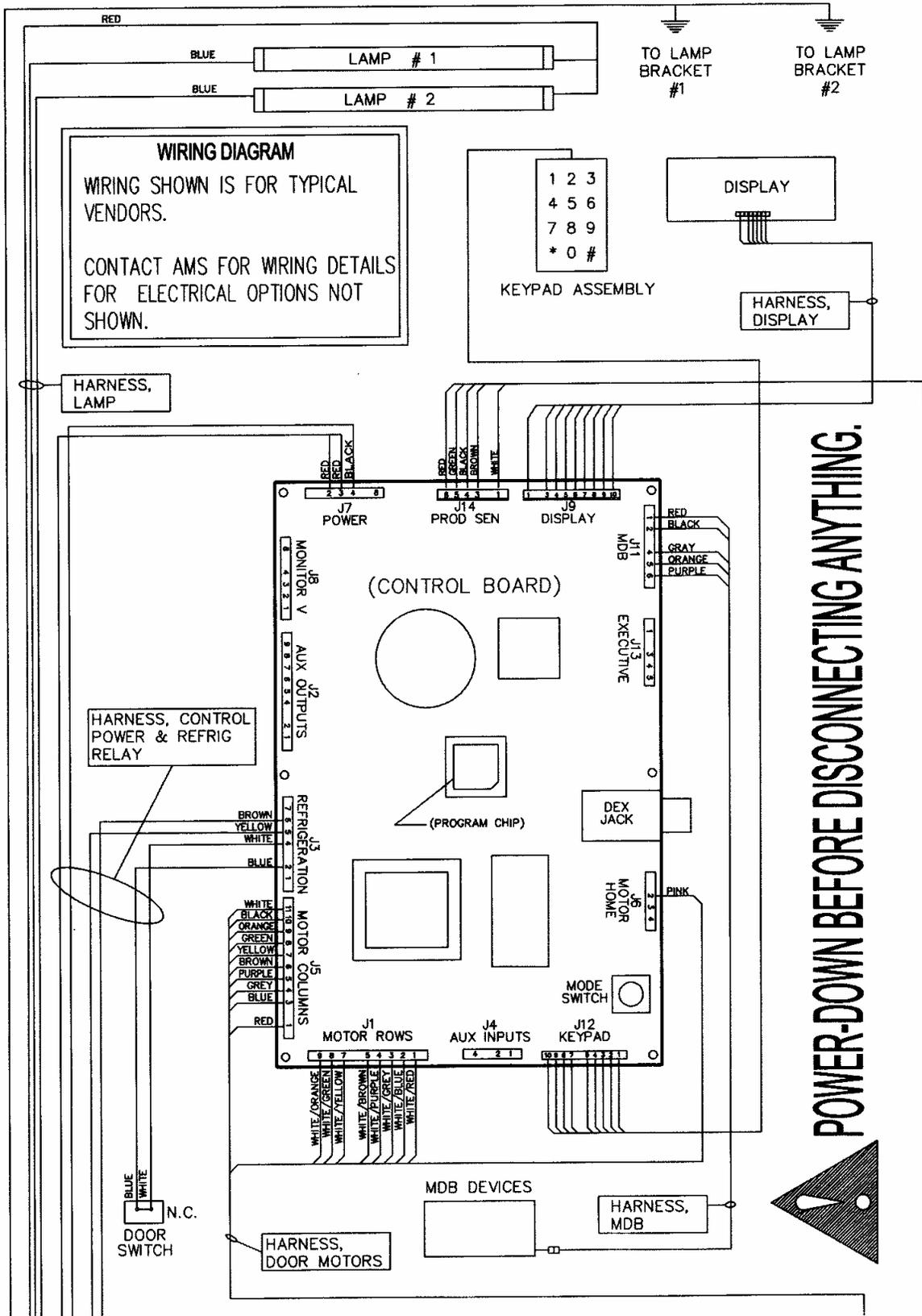
Figure 9.1 Typical Wiring Diagram, Sheet 1 of 4
