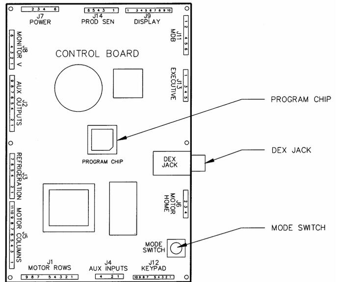
Figure 3.1 Control Board Components
