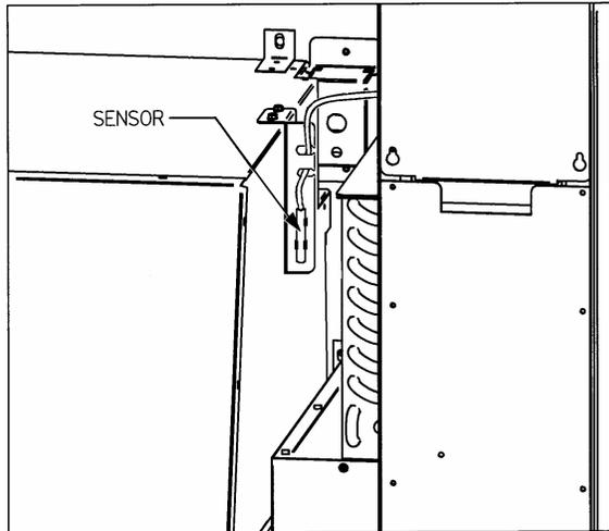
Figure 8.3 Temperature Sensor
